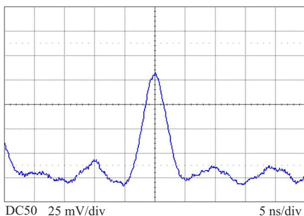
**Figure 3.** An oscilloscope of a dark count signal from a pixel with an amplitude of 4 photoelectrons.
