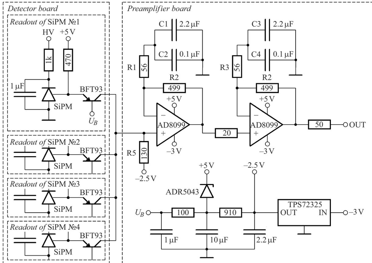
Figure 1. Simplified electric circuit of pixel.
