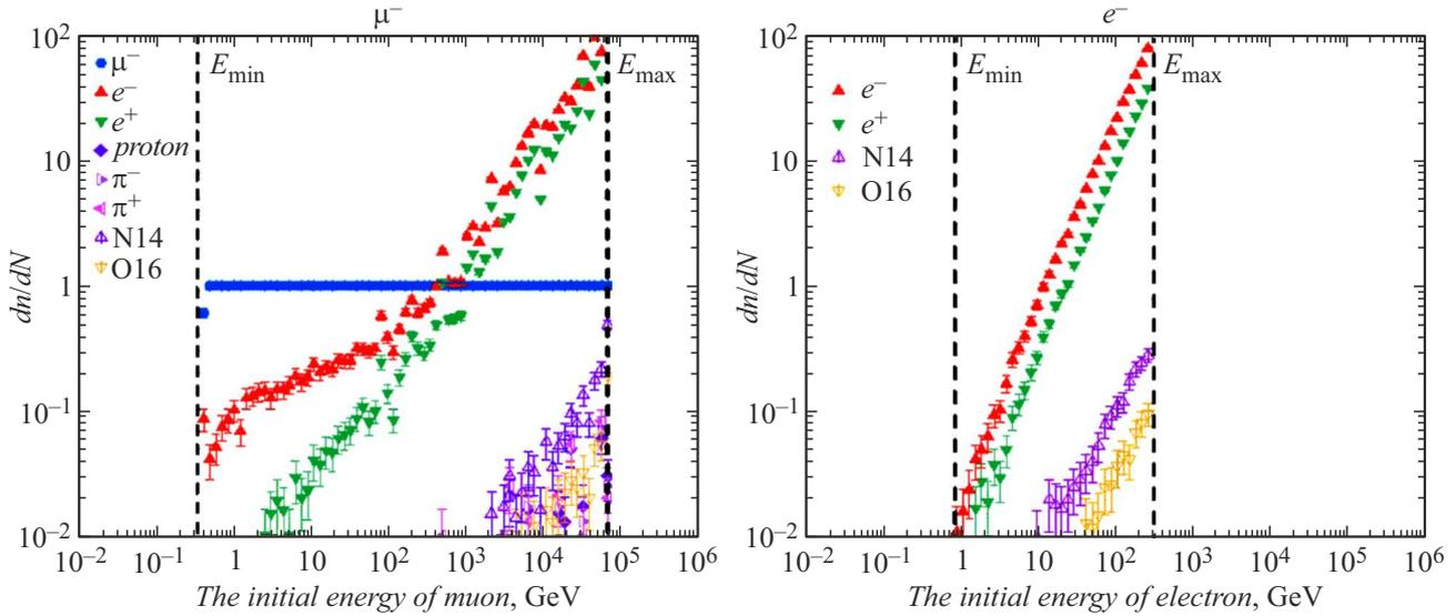
**Figure 2.** Number of charged particles ( $dn/dN$ ) that passed through the second drift chamber layer with respect to the initial number of particles depending on the energy of the initial particle: muon and electron.
