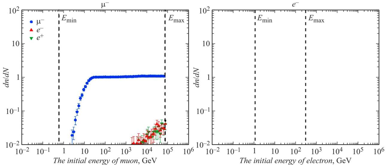
**Figure 3.** Number of particles reconstructed as a muon ( $dn/dN$ ) with respect to the initial number of particles depending on the energy of the initial particle: muon and electron on four drift chamber layers.
