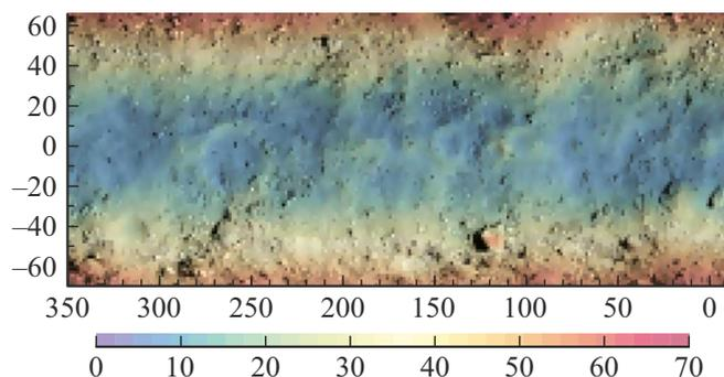
**Figure 2.** Benu map model [6]. On the latitude axis, the scale is given in degrees from  $+60^\circ$  to  $-60^\circ$ , on the longitude axis, the scale is given in degrees from  $+0^\circ$  to  $350^\circ$ . Color scale of heights above geopotential in meters is shown at the bottom of the figure.
