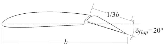
Figure 1. Computational model of the wing-flap profile .
