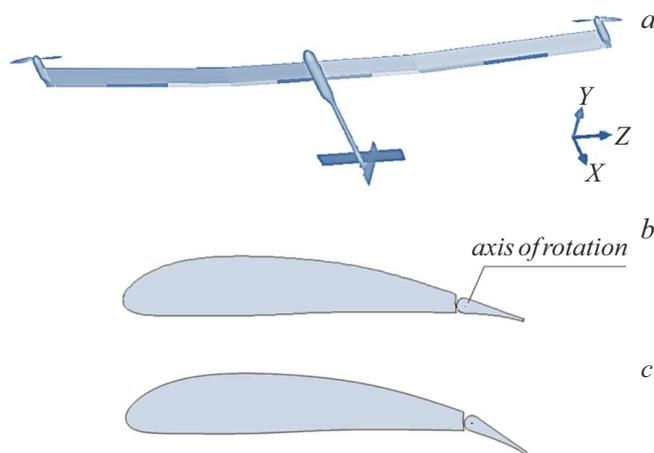
**Figure 1.** Design model of airplane: *a* — general view, *b* — wing section  $\delta = 0$ , *c* — wing section  $\delta = 15^\circ$ .
