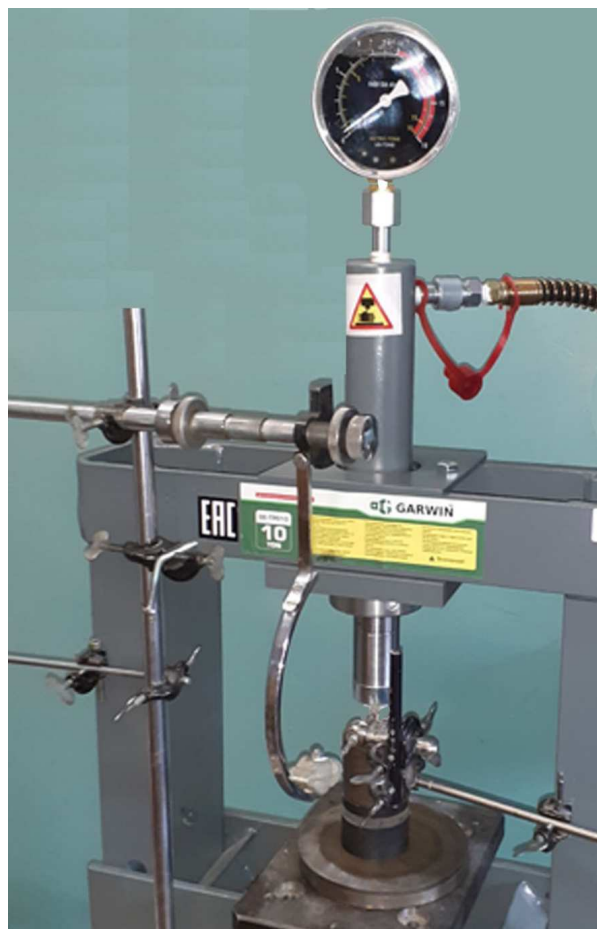
Figure 1. General view of a system for AE generation with impact damage of an uniaxially compressed CR sample.
