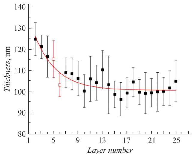
**Figure 2.** Dynamics of change in the thicknesses of high porosity layers in MC. The light-colored dots indicate the layers adjacent to the MC cavity layer.
