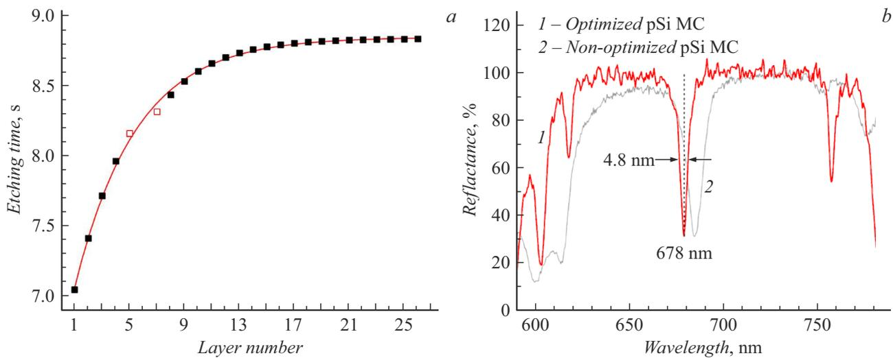
**Figure 3.** *a* — curve illustrating the corrections for etching times during fabrication of optimized MCs (light dots indicate the same as in Fig. 2). *b* — experimental reflectance spectrum of the optimized MC (1) compared with that of the unoptimized MC (2).
