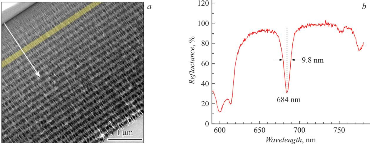
**Figure 1.** *a* — SEM image of the MC cross section. The arrow shows the direction of etching, the MC cavity is highlighted in yellow. *b* — reflectance spectrum of the unoptimized PS-based MC. A color version of the figure is provided in the online version of the paper.
