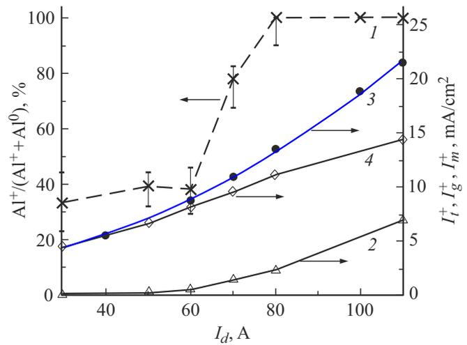
**Figure 3.** Dependence of the fraction of ions Al<sup>+</sup> in the vapor flow (1), pulse current density of metallic ions  $I_m^+$  (2), total ion current  $I_t^+$  (3) and gas ions  $I_g^+$  (4) on the discharge current amplitude. The average RPM current of the discharge is 12.6 A.
