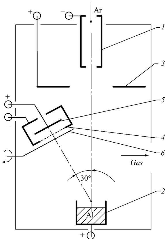
**Figure 1.** Experiment setup: self-heated cathode (1), crucible (2), auxiliary anode (3), two-electrode grid probe including grid (4) and collector (5), shutter (6).
