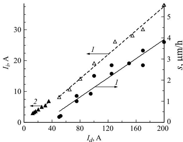
**Figure 2.** The dependence of the total ion current from the plasma  $I_t$  and the rate of aluminum film deposition  $s$  on the discharge current. 1 — in pulse-periodic mode, 2 — in continuous mode. The average discharge current is 12 A. In continuous mode,  $s = 0.5 \mu\text{m/h}$ .
