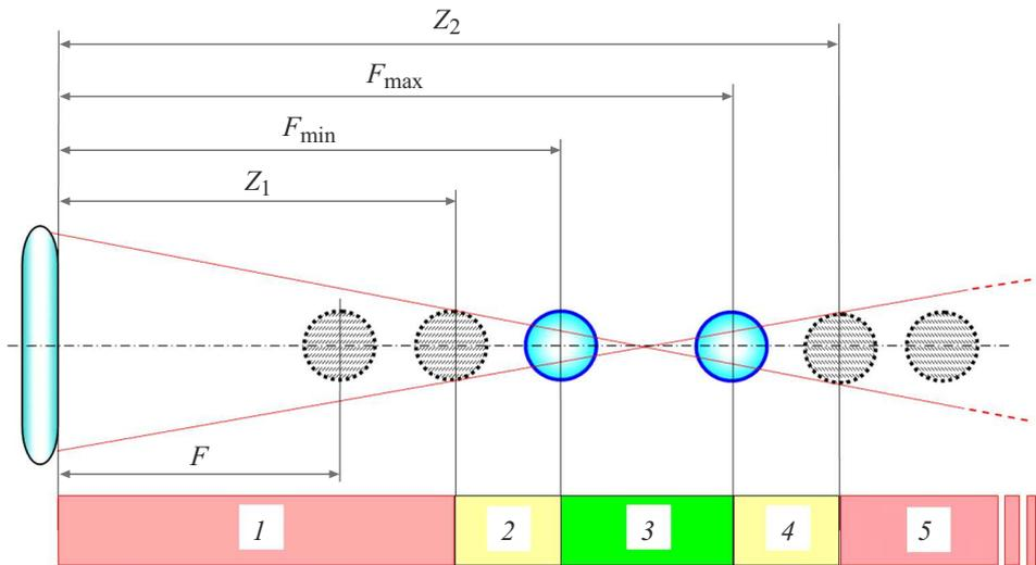
**Figure 1.** Classification of secondary sphere placement zones. 1 — zone of transit losses in the converging beam; 2, 4 — zones of increased optical losses of the extreme rays of the beam on the sphere surfaces; 3 — working zone; 5 — zone of transit losses in the diverging beam. A color version of the figure is provided in the online version of the paper.
