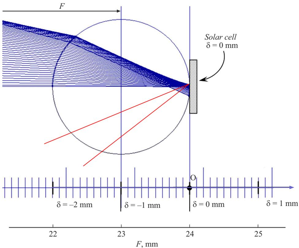
**Figure 2.** The path of the rays through the secondary optical element.  $\delta$  — distance from the top of the FBL output surface in the direction of ray path from POE,  $F$  — the focal distance of the lens. Rays experiencing total internal reflection at the sphere output surface are marked in red.
