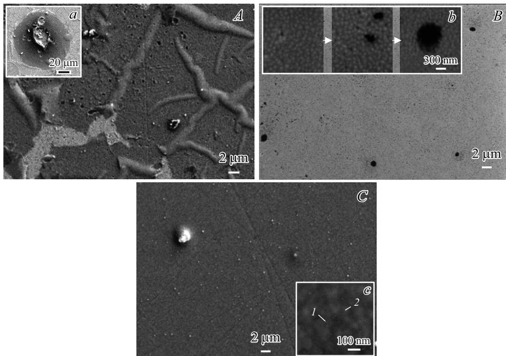
**Figure 2.** SEM image of the surface of samples A, B and C after testing. In insets: *a* — local rupture of the barrier structure with corrosion of the Ag layer; *b* — evolution of voids in the Ag layer with growth of grains; *c* — spherical particles (1) of size  $\sim 20$  nm at the grain boundaries of Ag (2).
