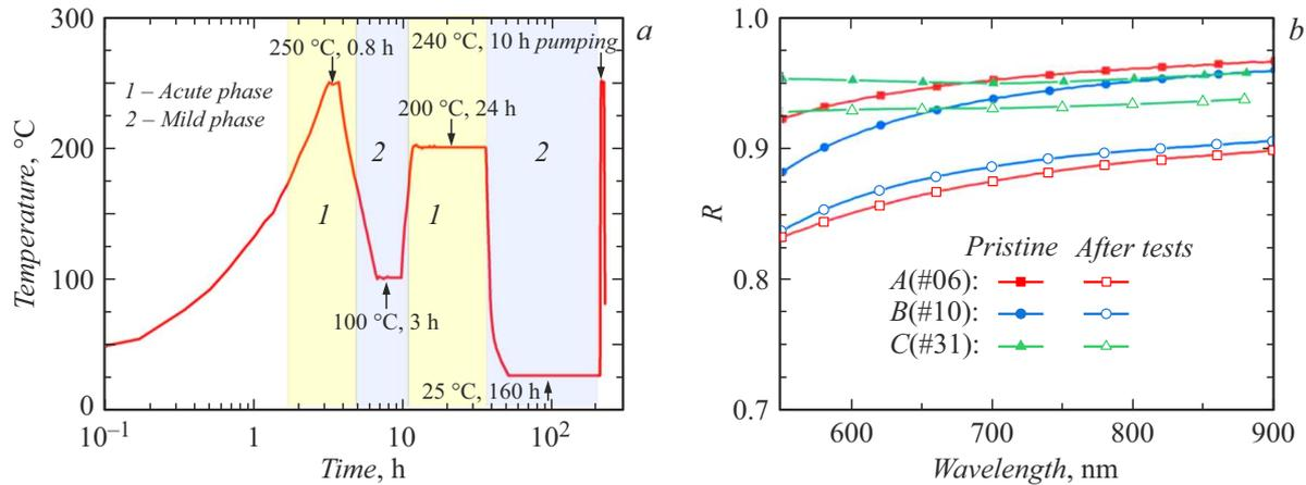
**Figure 1.** *a* — temperature profile of mirror exposure to water steam, simulating a steam ingress accident in ITER; *b* — spectral characteristic of the specimen specular reflectance of A, B, C before and after testing.
