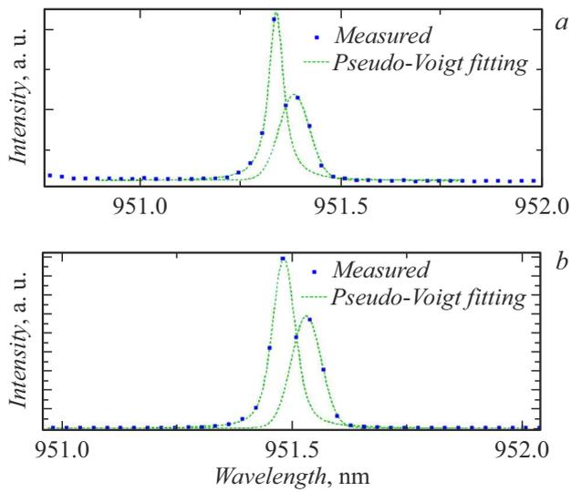
**Figure 1.** Generation spectra at 183  $\mu\text{W}$  (a) and 1.65 mW (b) optical pumping powers with the approximation result (dashed lines) for each peak (based on the pseudo-Voigt [9,14]).
