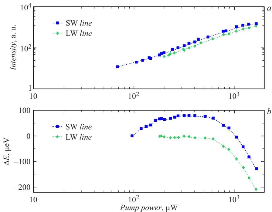
**Figure 2.** a — the dependence of the integrated emission intensity on the optical pumping power for modes with generation wavelengths of 951.34 nm (SW line) and 951.39 nm (LW line). b — the spectral shift of the position of the short-wave (SW line) and long-wave (LW line) modes with increasing optical pumping level.
