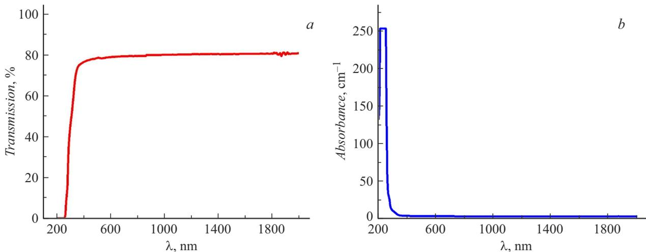
**Figure 2.** The optical characteristics of the sample  $\beta\text{-Ga}_2\text{O}_3\text{:Fe}$ . *a* — optical transmission spectrum, *b* — absorption coefficient.
