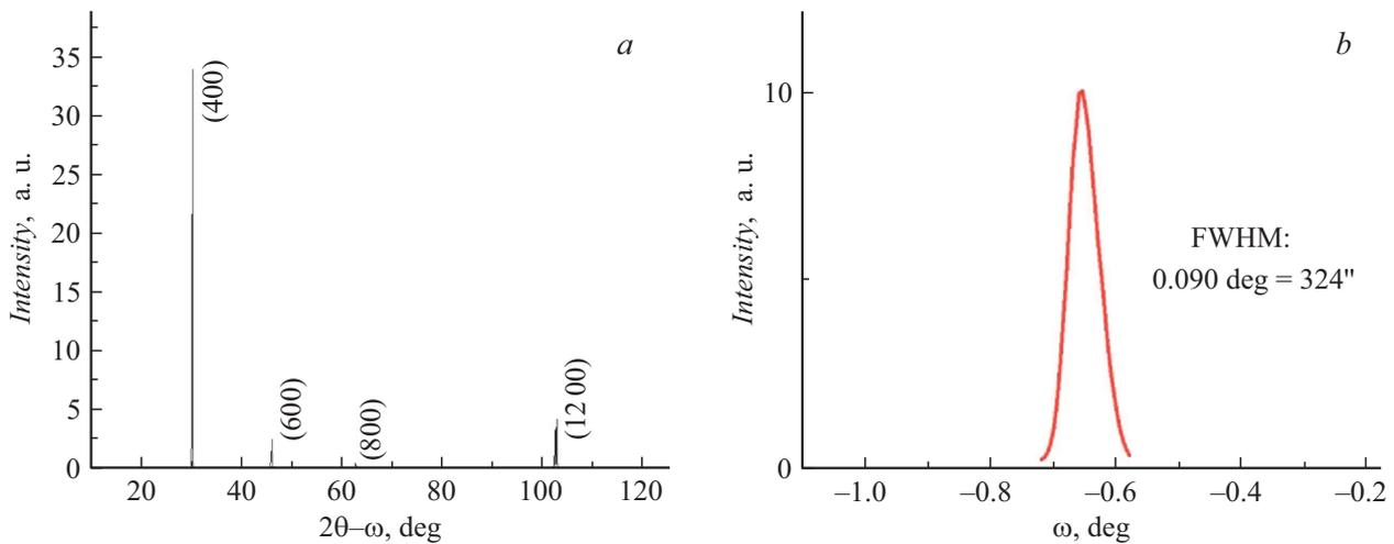
**Figure 1.** X-ray diffraction spectra of sample  $\beta\text{-Ga}_2\text{O}_3\text{:Fe}$ . *a* —  $2\theta\text{-}\omega$ -curve corresponding to the  $\beta$ -phase of gallium oxide, *b* — the swing curve for the reflection from the (400) plane.
