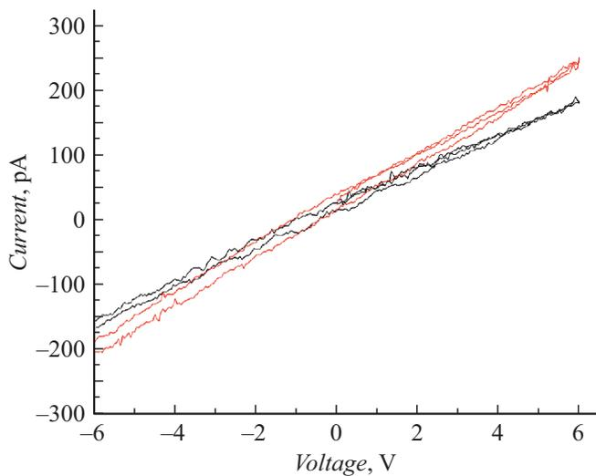
**Figure 3.** Volt-ampere characteristics obtained on a thin sample. The current direction was along the crystallographic direction [100].
