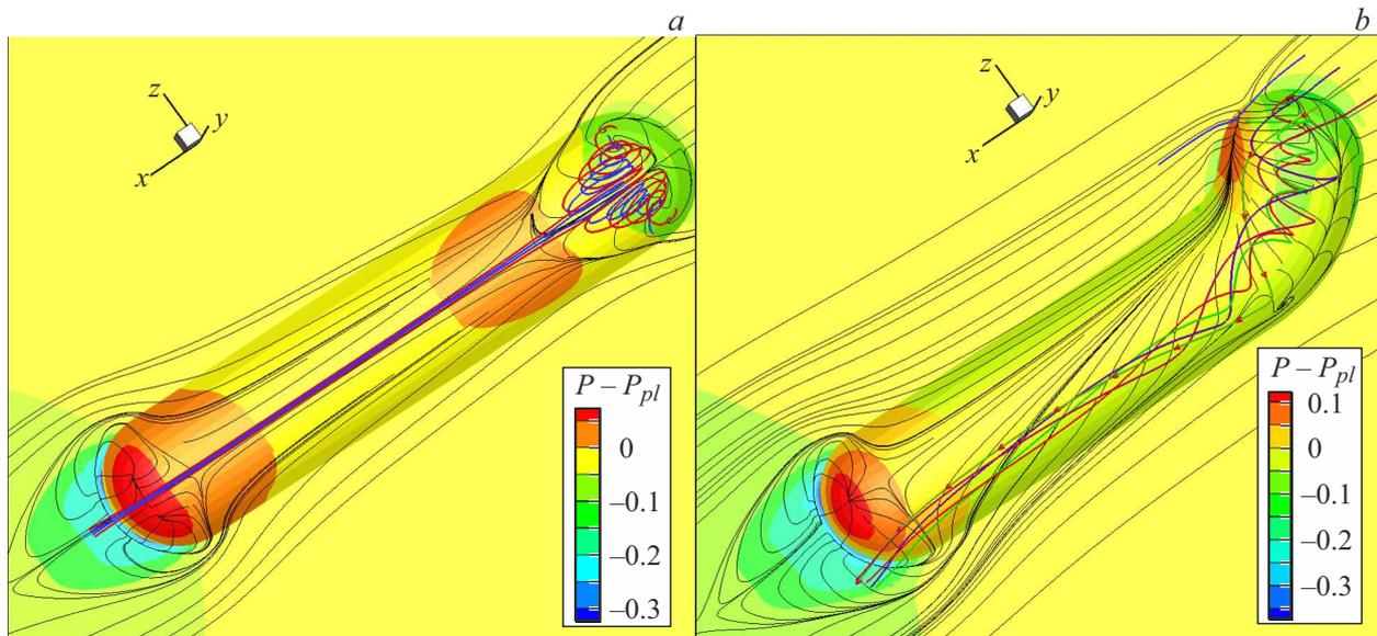
**Figure 1.** Surface fields of pressure drops  $P - P_{pl}$  in the longitudinally oriented groove (a) and deflected tip groove  $\xi = 0.15$  in relative length (b) with applied spreading patterns and spatial vortex structures.
