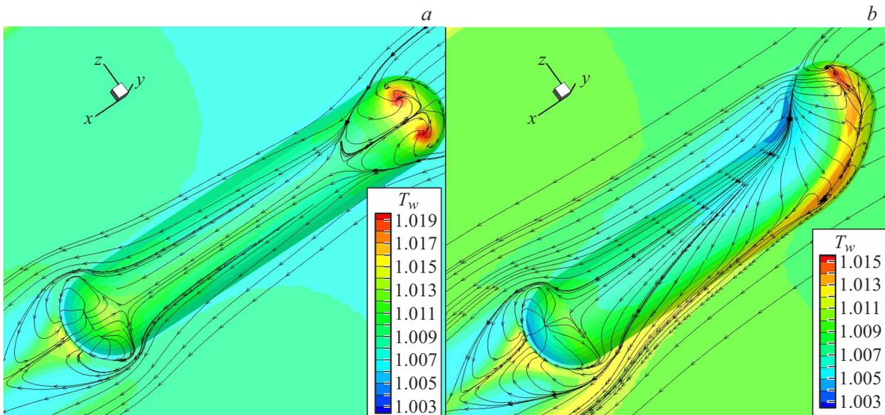
**Figure 3.** Surface temperature fields in the longitudinally oriented groove (a) and groove with the deflected tip having relative length  $\xi = 0.15$  (b) with applied spreading patterns.
