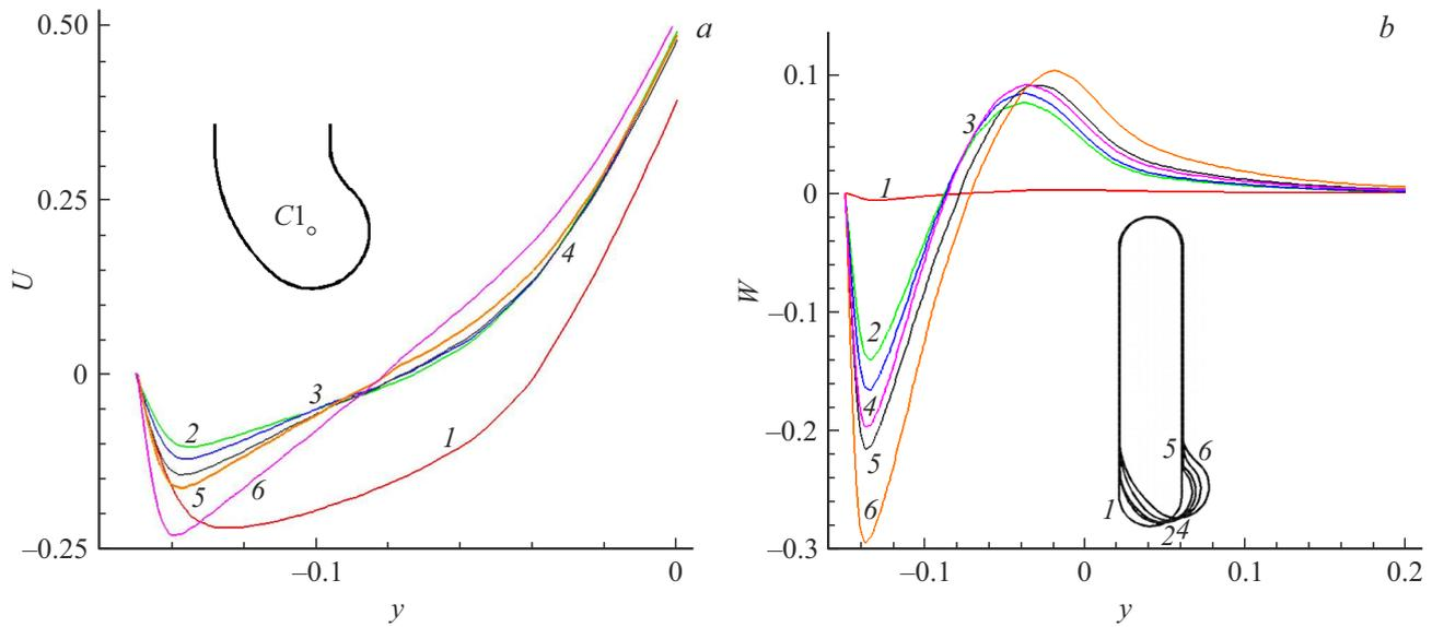
**Figure 2.** Comparison of profiles of the Cartesian longitudinal  $U$  (a) and transverse  $W$  (b) velocity components at different relative lengths of the grooves inclined tip  $\xi$  in the center of the crosssection of transition between the spherical segment and trench part  $C1$ .  $\xi = 0$  (1), 0.05 (2), 0.06 (3), 0.075 (4), 0.1 (5) and 0.15 (6). The figure depicts contours of the grooves under consideration.
