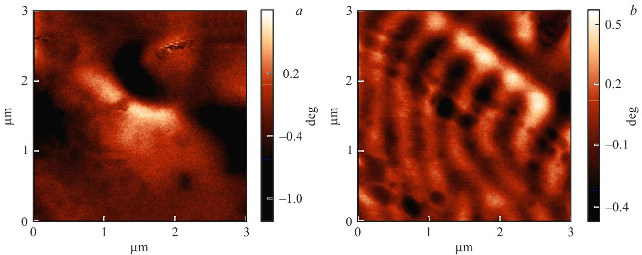
**Figure 1.** Magnetic phase contrast images of films *D* (*a*) and *G* (*b*). The right panel presents on the vertical color scale the phase shifts (in degrees) of oscillations of the cantilever with a magnetic probe. The colored figure is given in the electronic version of the article.
