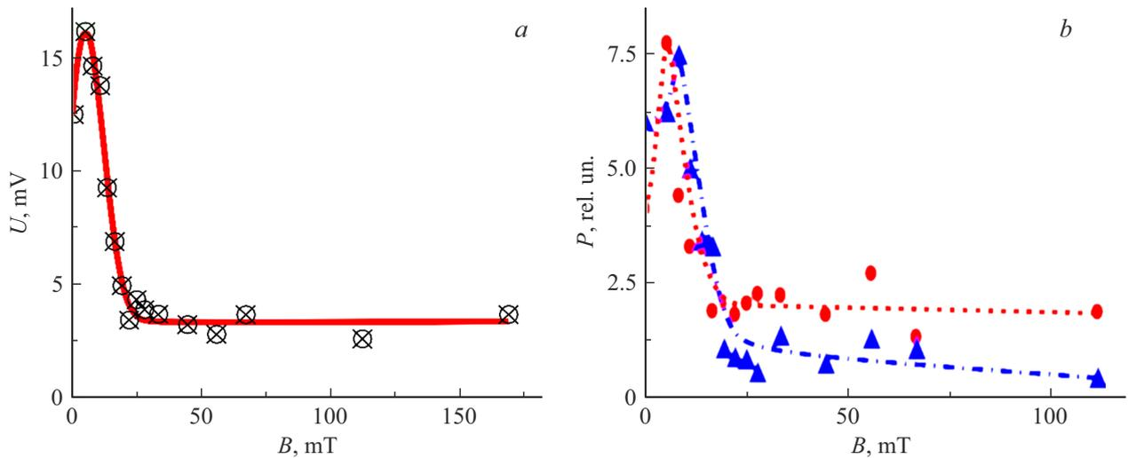
**Figure 3.** *a* — electric pulse amplitude dependence on magnetic field induction *B* for film *G*; *b* — dependences of the spectrum components power at the frequencies of 61 MHz (dotted curve) and 72 MHz (dash-dotted curve) for film *G*.
