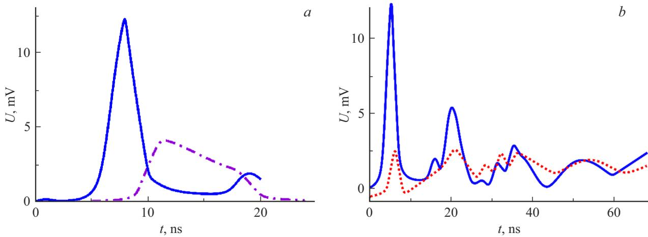
**Figure 2.** *a* — time dependences of the piezoelectric-transducer electric pulse amplitude for films *D* (dash-dotted curve) and *G* (solid curve) in the zero magnetic field; *b* — time dependences of the electric pulse amplitude for film *G* in the absence of magnetic field (solid curve) and in magnetic field of 0.2 T (dotted curve).
