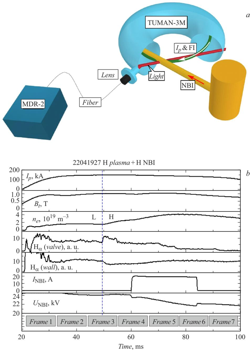
**Figure 1.** *a* — optical measurement system; *b* — time evolution of the discharge parameters. Top-to-bottom: plasma current, toroidal magnetic field, mean chord central density,  $H_\alpha$  line emission near the gas puffing valve and near the wall, NBI pulse, CCD-camera frames. NBI energy is  $W_b \sim 22$  keV, beam current is 19 kA.
