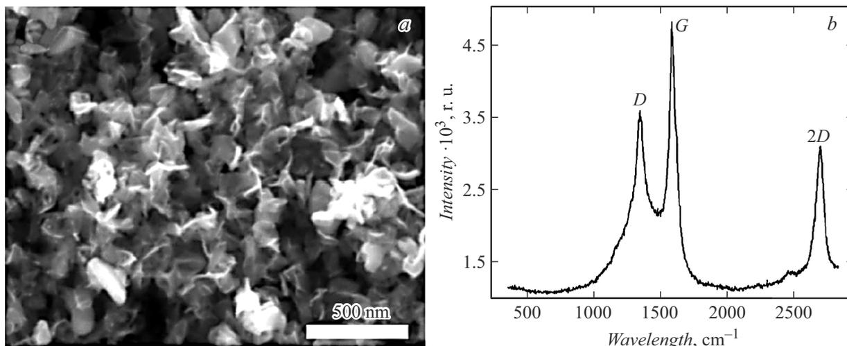
**Figure 1.** SEM image (a) and RS spectrum (b) of multi-graphene nanoparticles synthesized during conversion of mixture  $C_3H_8-C_4H_{10}/He$  with the ratio of 0.05/0.75 g/s accordingly. Current — 400 A, pressure — 500 Torr.
