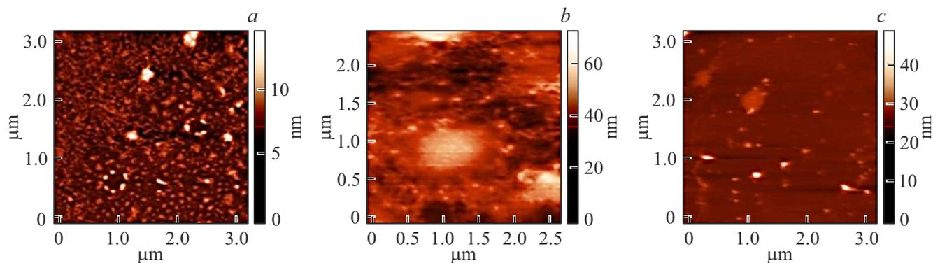
**Figure 3.** Films from single-component suspension from cyanobacteria: *a* — single application of suspension, *b* — triple application of suspension, *c* — printed film of four layers.
