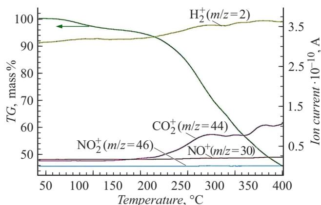
**Figure 4.** Thermal analysis of film from cyanobacteria.
