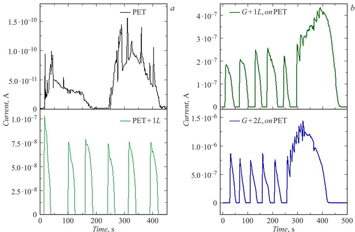
**Figure 5.** Responses to breathing (a) for PET (upper part of the drawing, PET) and layer of cyanobacteria on PET (lower part of the drawing, PET+1L) (b) for the layer of cyanobacteria on the structure of CVD-graphene/PET (upper part of the drawing, G + 1L, on PET) and two layers of cyanobacteria on the structure of CVD-graphene/PET (lower part of the drawing, G + 2L, on PET). Voltage applied to the structure when recording the characteristics was 1 V.
