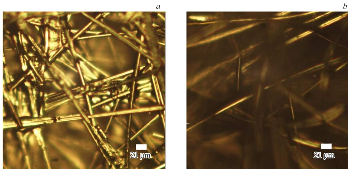
**Figure 7.** Optical image of carbon fibers without (a) and with addition of suspension from cyanobacteria (b).
