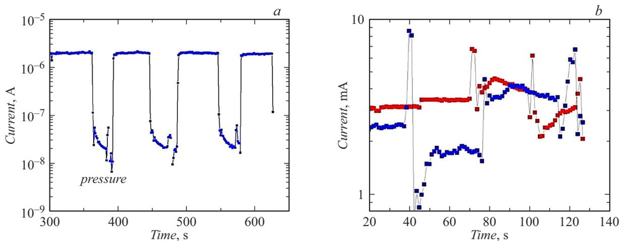
**Figure 9.** Change of current in time when pressed for carbon fiber with addition of cyanobacteria (a). Response to pressing from two sensors from multigraphene synthesized in plasma with addition of cyanobacteria and Nafion (b). The applied voltage was 1 V.
