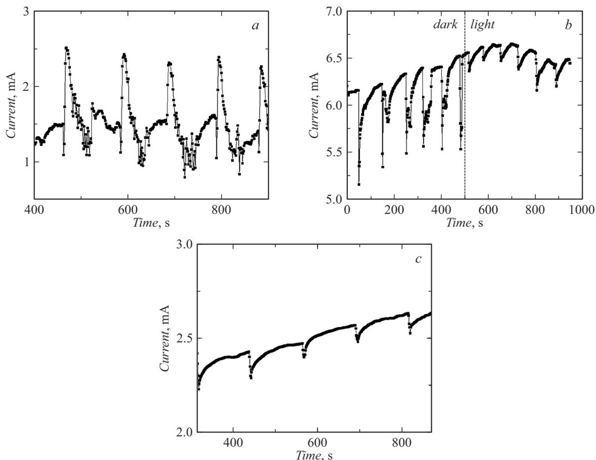
**Figure 8.** Response of carbon fiber to breathing (a). Carbon fiber response to breathing with addition of cyanobacteria with and without lighting (b). Carbon fiber response to breathing with addition of a layer of cyanobacteria and Nafion polymer mix (c). Voltage applied to contacts was 0.1 V.
