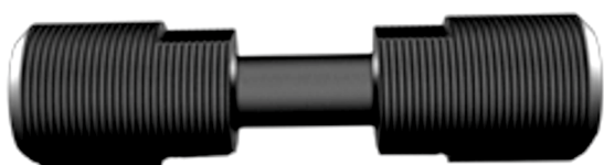
Figure 2. Tension sample for tests in HSR.
