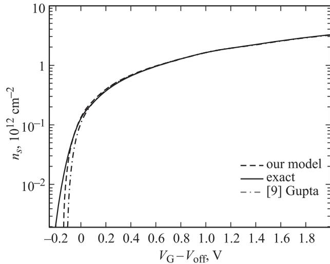
**Fig. 3.** Variation of sheet carrier concentration ( $n_s$ ) with applied gate voltage ( $V_G - V_{\text{off}}$ ) at 300 K: solid line (exact), dashed line (our model), chain-dotted line Gupta [9].
