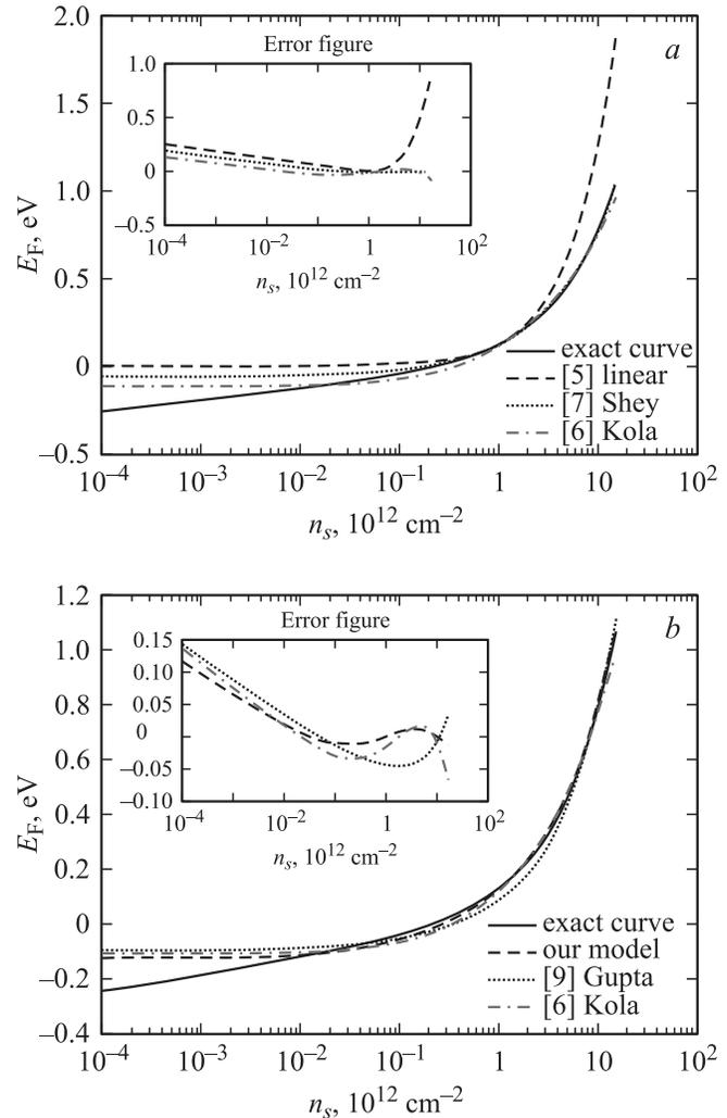
**Fig. 1.** Variation of the Fermi potential ( $E_F$ ) with sheet carrier concentration ( $n_s$ ) at 300 K.
