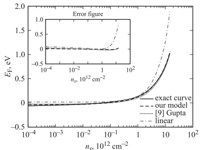
**Fig. 2.** Variation of the Fermi potential ( $E_F$ ) with sheet carrier concentration ( $n_s$ ) at 77 K: solid line (exact), dashed line (our model), dotted line [9], chain-dotted line (linear).
