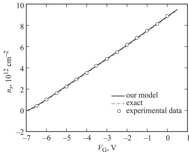
**Fig. 4.** Measured and simulated sheet carrier density versus the gate bias. The barrier thickness  $d = 35$  nm and the threshold voltage  $V_{\text{off}} = -6.78$  V.
